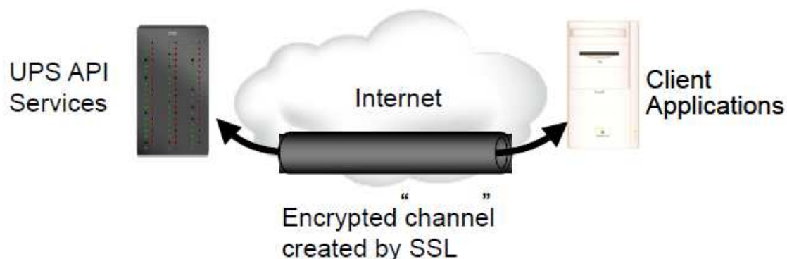
Figure 2: SSL creates a secure channel across a network and protects confidential communications using that channel.
