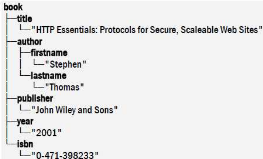
Figure 9. It is possible to show the tree-like structure of XML messages using text.
